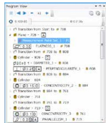
MiCAT Planner prevents from any misinterpretation risk: each GD&T symbol, tolerance and datum is automatically understood and converted in the corresponding required measurement points. In the program view, all GD&T are shown in regards to the feature to be measured for calculating the result.
