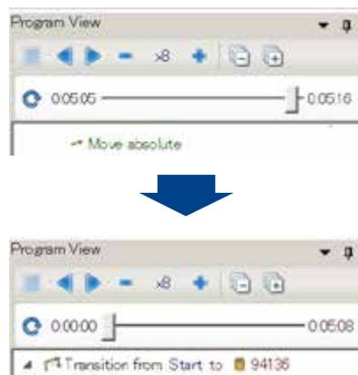
Furthermore, MiCAT Planner automatically estimates the measuring cycle time according to the actual CMM configuration and settings. For example, the required time for exchanging a probe in the rack, or the specified scanning speed in your measurement rules are considered for this time estimation. Immediately after the cycle optimisation calculated, the estimated new cycle time is displayed.
