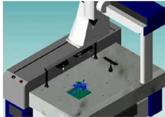
MiCAT Planner selects the best-suitable probe configuration for each feature under consideration of the customised measuring rules.
