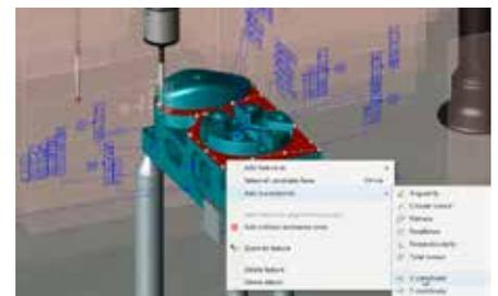
If required, a missing feature (not identified on the CAD model) or a missing characteristics to be evaluated can be manually added from the 3D view.
