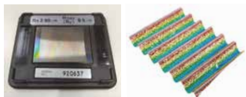
Specimen rugozitate 3 \mu\text{m}
