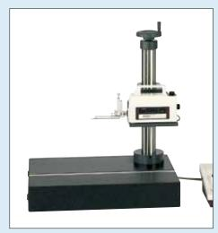
The SJ-500 can also be mounted on a manual column stand.
