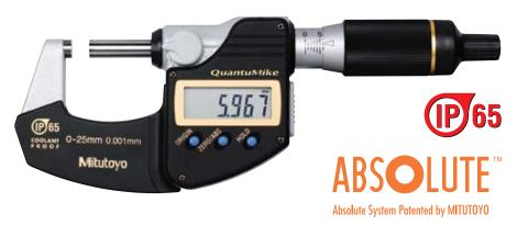
Conventionally, a digital micrometer leadscrew needs a fine pitch, typically 0.5 mm, to give enough mechanical magnification for the miniature rotary encoder on the spindle to achieve the required resolution. This makes the micrometer slow to adjust when taking measurements and checking the origin point. This is frustrating for the user and is a factor that limits measurement efficiency.
