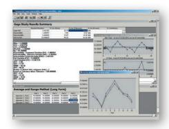
In addition to the standard calculations this software also provides graphical tools for analysis of the measurement system. The Xbar and R chart can show whether there is adequate gage discrimination to record part to part variation in production and if operators are self-consistent. The Part-by-Appraiser plot can show if there is a lack of consistency between operator inspection techniques.
