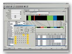
MeasurLink Gage Management allows customers to build a complete gage (and fixture) inventory. Calibration procedures are established using a sequence of Standards. These procedures are associated with Gage IDs and are used when performing "in-house" calibration.
